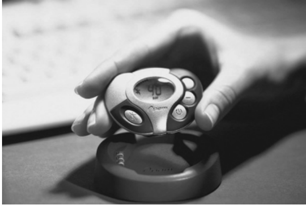
Fig. 1. Personal Activity Monitor (PAM) with reader interface unit.
